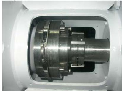
The Pellermix seal Isolation device work through a plug and seal design. The device allows for the seal change whilst the tank is full.
